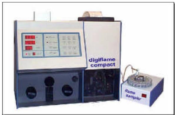
**AUTOMATIC FLAME ANALYZER for the simultaneous determinations of Sodium (Na) Potassium (K) and Lithium (Li) on serum, urine or different samples, with built-in 1:100 peristaltic diluter and data printer**
